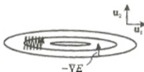
Figure 2.9: Schematic illustration of fixed-step gradient descent for an error function which has substantially different curvatures along different directions ([Bishop, 1996, p. 265]).
